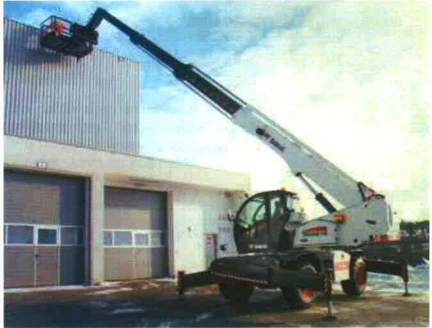
Right: With a Bobcat man platform attachment the Bobcat TR50210 Rotary Telescopic Handler transforms into an aerial work platform.
