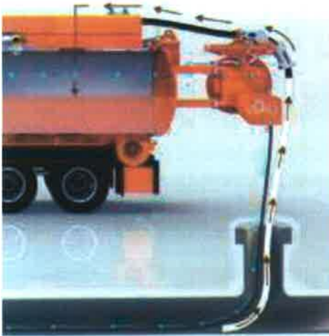
Above: Purpose-built for cleaning sewage and storm water drains, the HPVR-1000's recycling system recaptures water for re-use in the jetting process.
