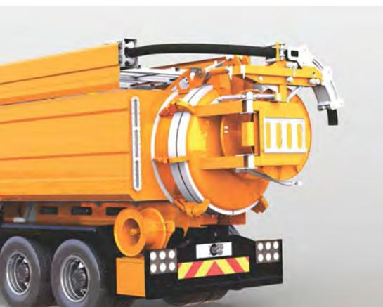
vacuum and jetting systems on standard truck chassis homologated for on-road use in Southern Africa. "The new Mobile Vacuum Trailer is a direct result of our close cooperation and team work with Highpoint Vacuum. This machine meets the need that we identified in the market for an easy to set up and manoeuvre machine for plant clean-ups."
